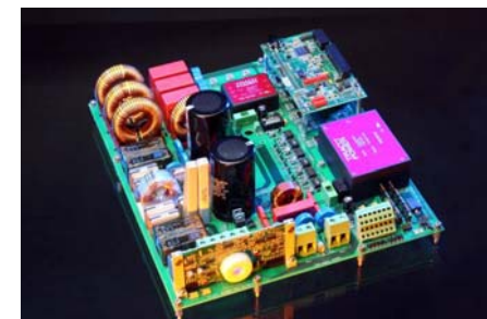
Motherboard of the 6.9 kWp Tracking Inverter
