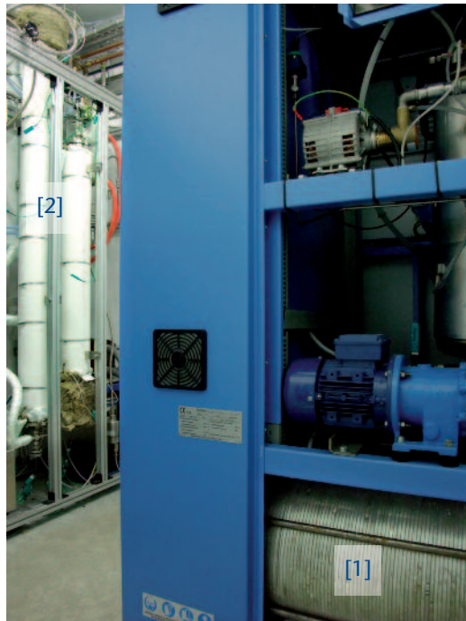
Figure 4 Container-integrated wind to SNG system with electrolysis stack [1] and methanation device [2]
