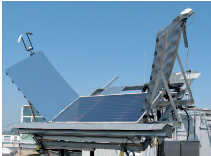
Figure 2 Second test sample of the RefleC collector for measuring the efficiency curve at Fraunhofer ISE (rotated 90 ° counter-clockwise).
