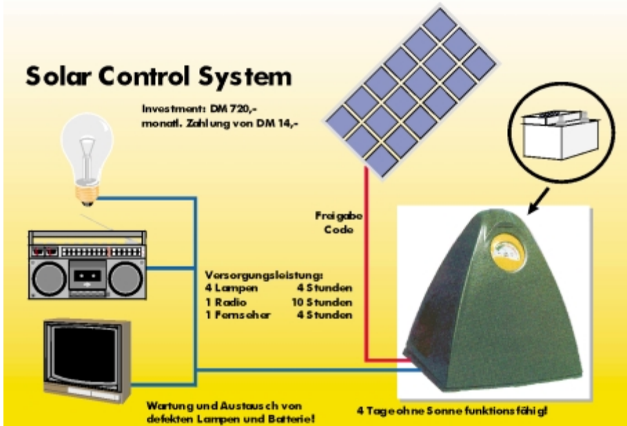
Abbildung 5: Solar Control System
