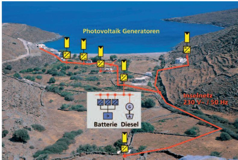
Stand-alone grids can be connected to one another or to the integrated grid using suitable, i.e. grid compatible control technology. This allows so-called micro-grids to be formed temporarily, which can then continue to operate without problems even if the main grid fails (Figure 7).
