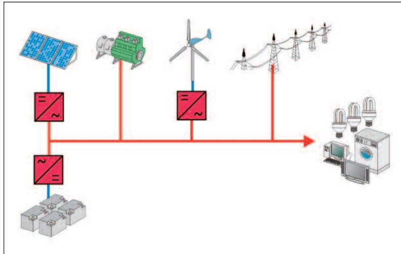
Hybrid systems can be designed as DC systems, mixed DC/AC systems or pure AC systems. DC/AC systems are often used in farms or other small companies. When designing systems, planners must take into account that the inverter power must match the overall maximum consumer power. **Mixed DC/AC systems** are particularly suitable for combining medium AC loads with DC generators. At the same time, this also allows the battery on the DC side to be charged via a combustion generator (Figure 2).
