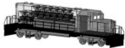
Conceptual design of a fuel cell engine applying 1.2 MW PEM fuel cells (blue) and six sets of 280 kW of hydrogen as a separate fuel to drive a turbine
