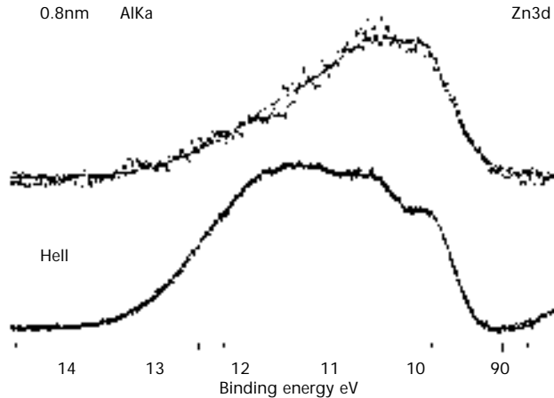
Figure 3 Hell and AlKa spectra of the Zn3d emission for a very thin ZnO film (.8nm). The observed structure is directly rela- ted to the complex inter- face morphology
