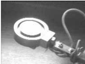
Figure 1 A schematic sketch and a photograph of the thermal probe.
